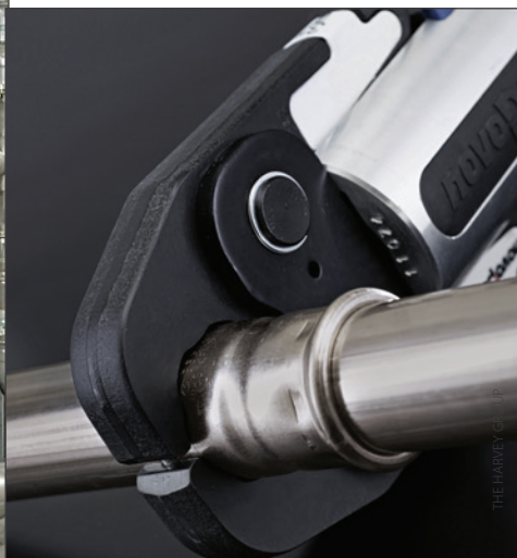
▽ Pressfitting being sealed onto piping using an electro-mechanical pressing tool. The pipe and pressfitting diameters span from 15 to 108mm diameter for this system. The fittings feature a blue pressing indicator that is removed as part of the correct pressing procedure so that any missed joints can be quickly identified.
